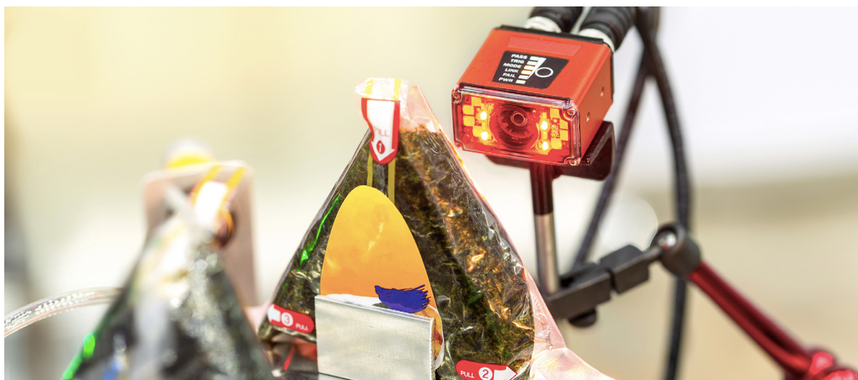
Barcode-reading technology on a sushi industrial production line.
